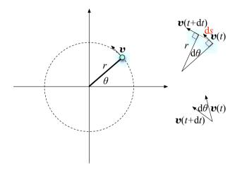
We consider the weight connected to a string is rotating around the origin at a constant velocity v. The velocity v is always constant, so the force should be perpendicular to the velocity. The force is given by the the string tension. The acceleration **a** is given by
