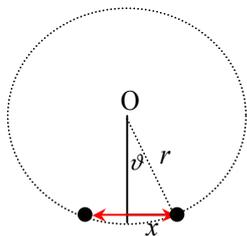
$$m \frac{d^2 x}{dt^2} = mr^2 \frac{d^2 \vartheta}{dt^2} = -kr\vartheta \Rightarrow I \frac{d^2 \vartheta}{dt^2} = -\tau\vartheta$$
