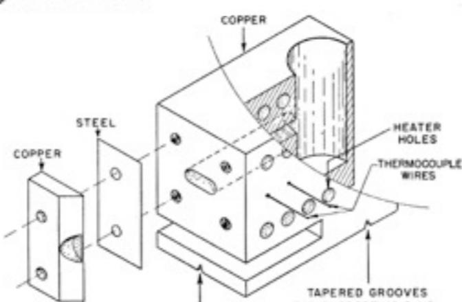
FIG. 3. Copper oven used for potassium showing details of slit construction.
