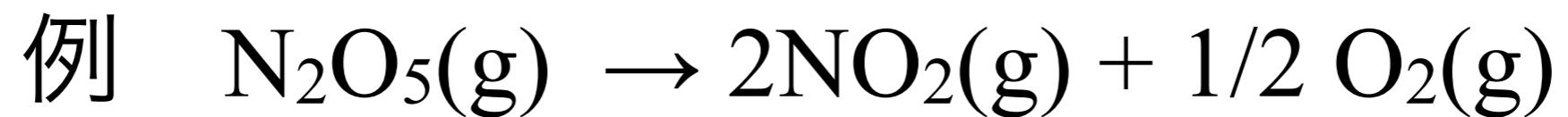
$$\nu(t) = -d[\text{N}_2\text{O}_5]/dt = k[\text{N}_2\text{O}_5]$$
