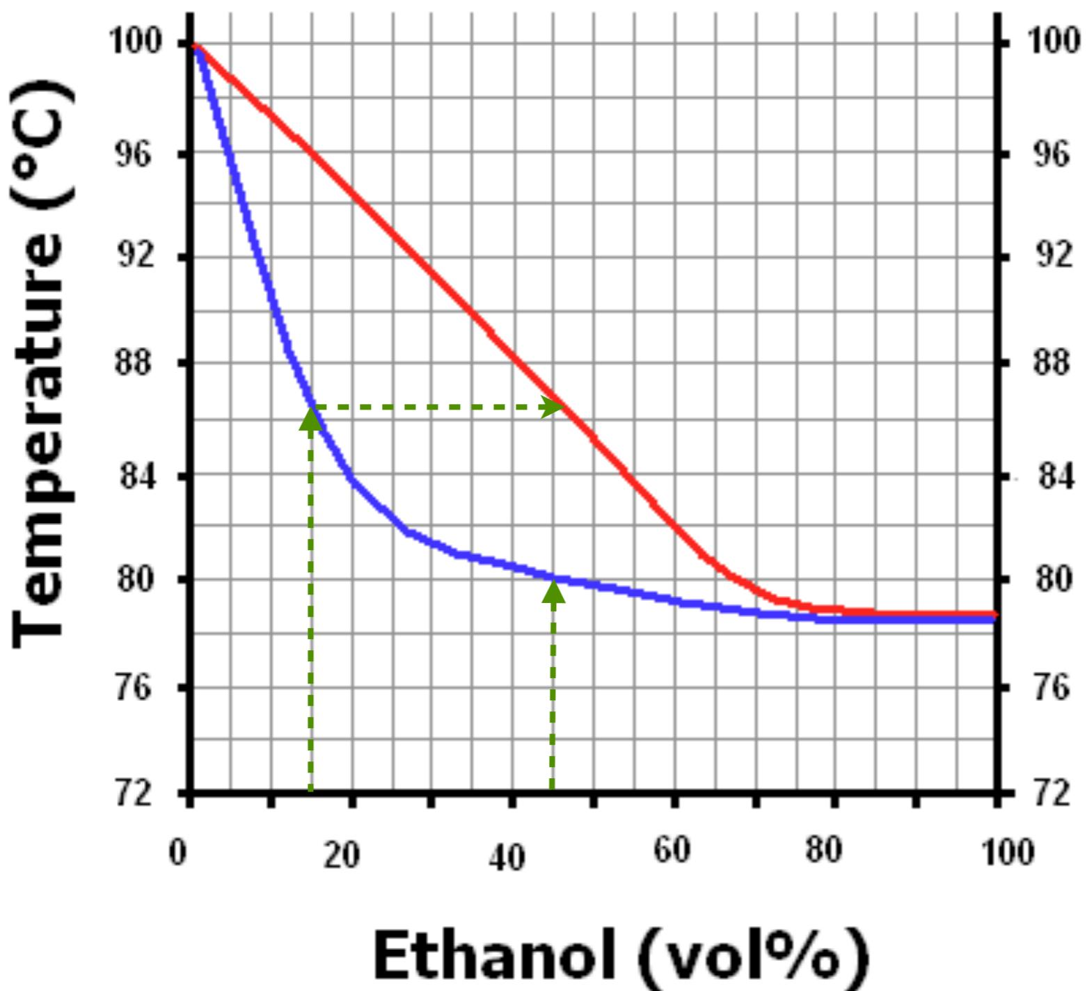
A phase diagram (NOTE: VERY INACCURATE DATA) representing the boiling point of a mixture of ethanol and water, and the composition of the vapour phase.
