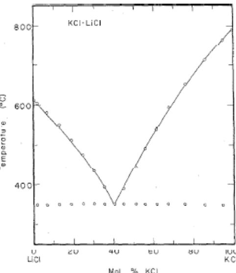
FIGURE 68. Temperature composition phase diagram for KCl-LiCl.
